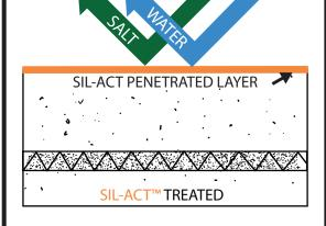
**SIL-ACT**®'s penetrated silane treatment layer stops water and salt intrusion into concrete, brick, masonry and many types of stone without affecting natural vapor permeability.
