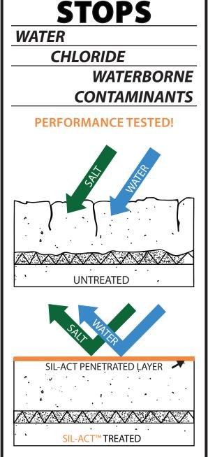
SIL-ACT<sup>®</sup>'s penetrated silane treatment layer stops water and salt intrusion into concrete, brick, masonry and many types of stone without affecting natural vapor permeability.
